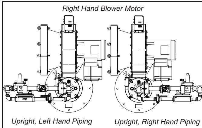
**Figure 3.1 Burner Configuration & Motor Orientation Choice**
